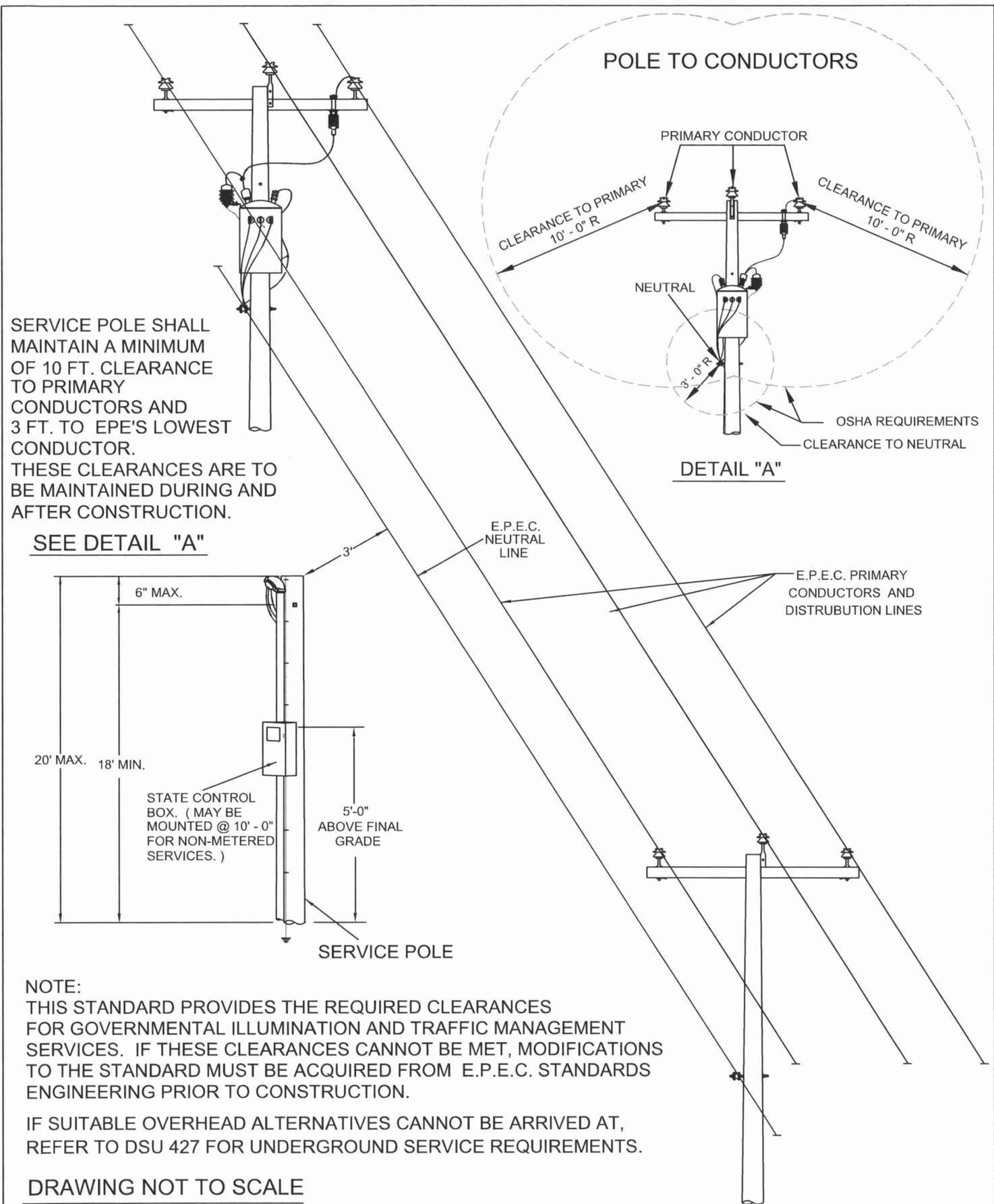
SERVICE POLE SHALL MAINTAIN A MINIMUM OF 10 FT. CLEARANCE TO PRIMARY CONDUCTORS AND 3 FT. TO EPE'S LOWEST CONDUCTOR. THESE CLEARANCES ARE TO BE MAINTAINED DURING AND AFTER CONSTRUCTION.
